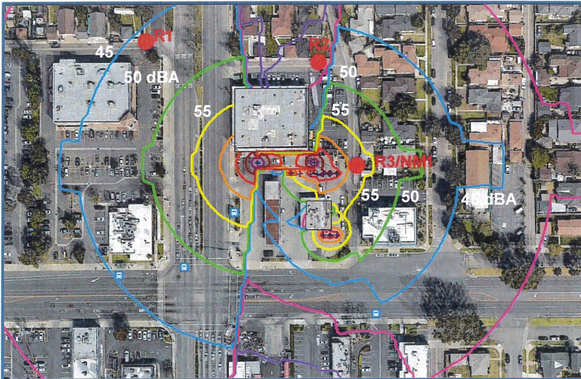
Figure 5. Noise Contour Map of the Future Car Wash Operations - Worst Case without Noise Control
