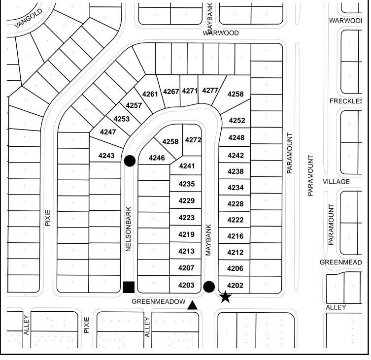
2 FULL CLOSURE POINT "ROAD CLOSED" 1 ADVANCED WARNING "ROAD CLOSED AHEAD" 1 "NO RIGHT TURN" 6 BARRICADES 1 "NO LEFT TURN" 8 DELINEATORS
