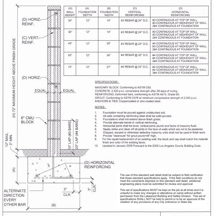
City of Lakewood Standard Wall Detail "G" Non-Retaining, Free Standing Condition, Between Two Private Properties T-Footing, 30" to 72" Above Grade SCALE: 1" = 1'-0"
