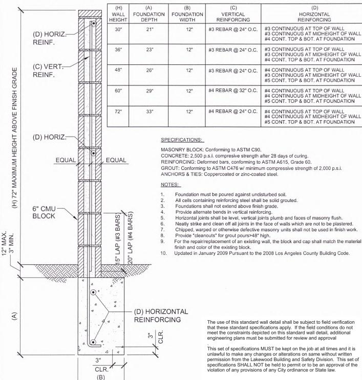
City of Lakewood Standard Wall Detail "H" Non-Retaining, Free Standing Condition, Between Two Private Properties I-Footing, 30" to 72" Above Grade SCALE: 1" = 1'-0"
