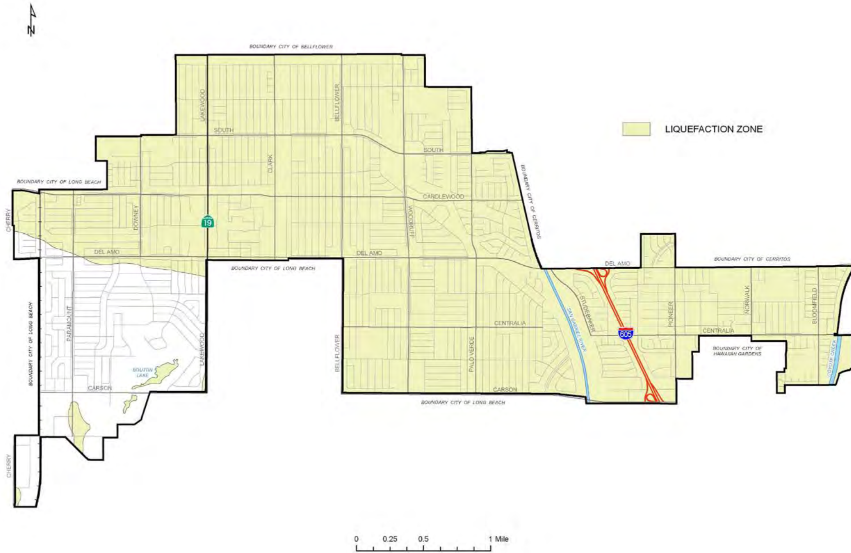
Figure 6-6: Areas with Potential Liquefaction in Major Earthquakes
