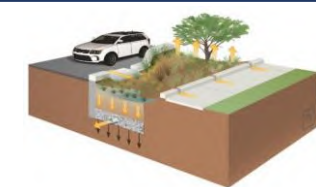
Bioretention w/ Underdrain
