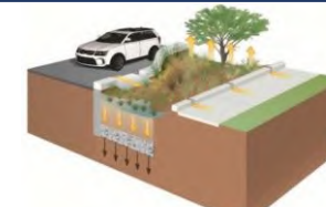
Bioretention w/o Underdrain
